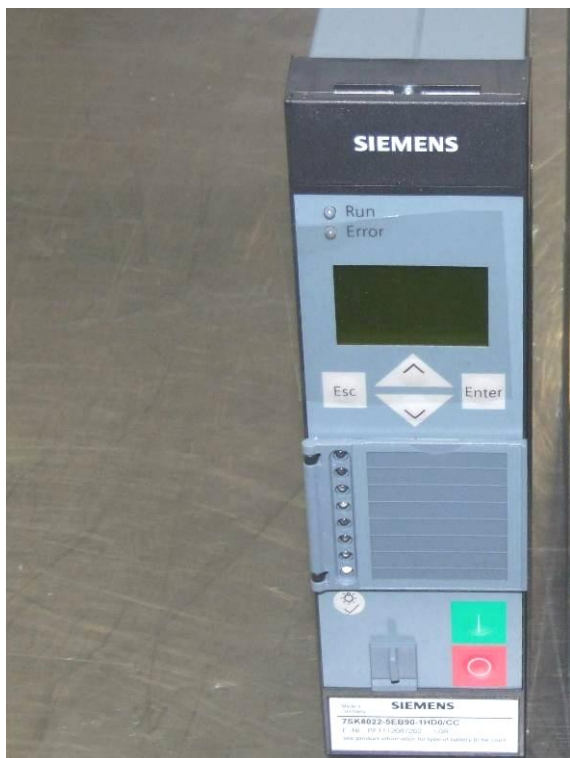
picture 1 Protection Relay 7SK80 before the corrosive test Ke
